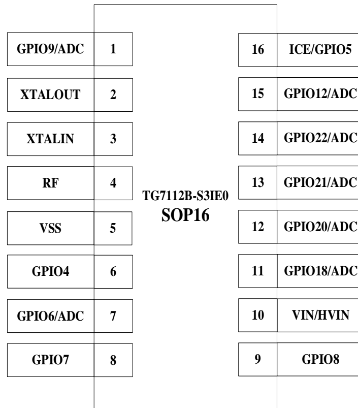
Figure 2-1 Pinout top view (SOP16 package)
