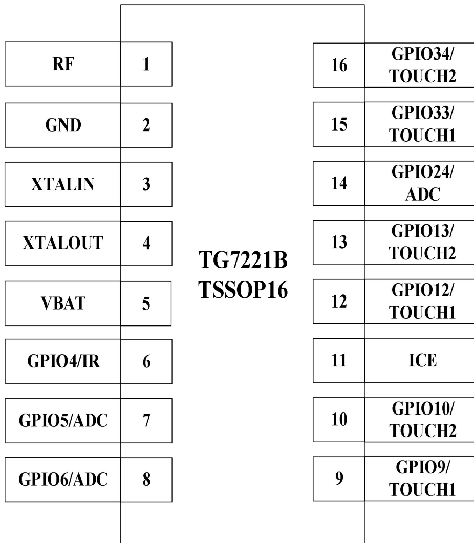
Figure 2- 1 Pinout top view (TSSOP16 package)
